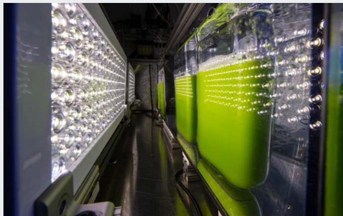
Photobioreactor used for carbon uptake and composition modeling. Photo by Dennis Schroeder, NREL 25505
